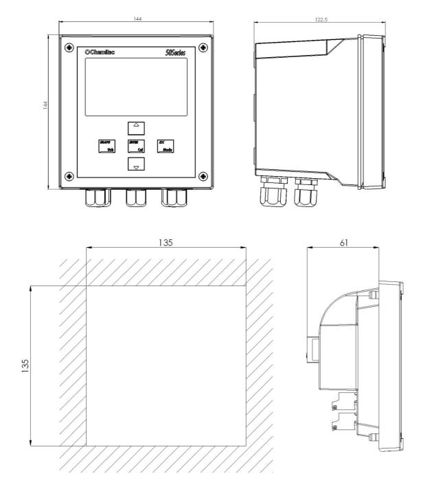
Dimensions (L x H x P) Mounting thickness Material Mounting Weight Front Panel I 44x I 44x I 22.5mm I 22.5mm Red ABS "RED 65" CIELAB Wall I Kg UV Resistant Polycarbonate
