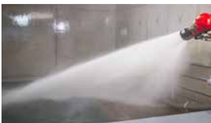
Flat jet with a modified spraying angle (special version)
