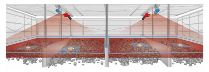
If a hotspot is detected in one of the sectors, it is extinguished in the hotspot area. (A monitor can cover several sectors as long as there is no shadowing by e.g. walls or pillars)
