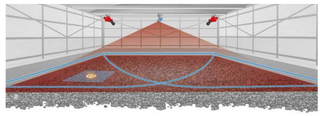
If a hotspot is detected in one of the sectors, extinguishing takes place in the hotspot area. (The camera controls the corresponding monitor).
