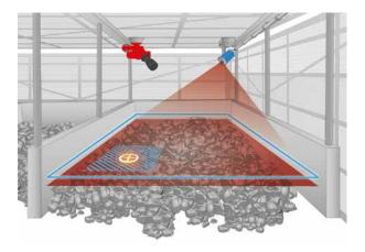
If a hotspot is detected extinguishing takes place in the hotspot area.
