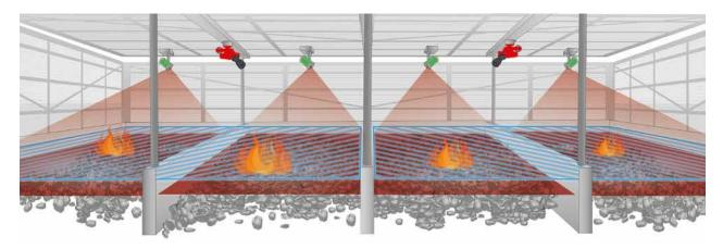
If a flame is detected in one of the sectors, the sector is extinguished.
