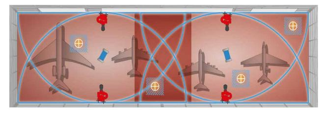
If a hotspot is detected in one of the sectors, extinguishing takes place in the hotspot area. (The camera controls the corresponding monitor).
